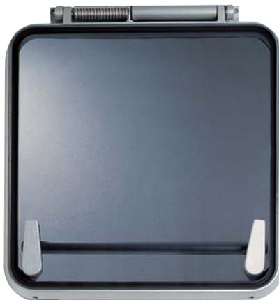
Escape hatches are used on multihulls and must be made open from inside and outside in case the boat capsizes. A locking bar prevents access from outside when moored. Using it when sailing is strictly forbidden. Homologation standards changed in 2002 for boats below 12 m (ISO/FDIS 12216/2002).
